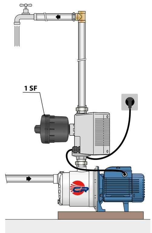
N.B.: It's advisable to install a membrane EXPANSION TANK (1SF) downstream of the inverter to:
