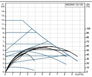
Pumped liquid = Water Liquid temperature during operation = 60  $^{\circ}$ C Density = 983.2 kg/m³
