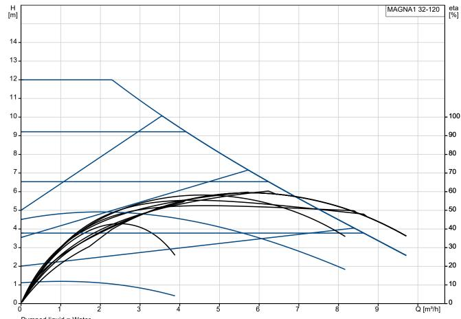
Pumped liquid = Water Liquid temperature during operation = 60 °C Density = 983.2 kg/m³
