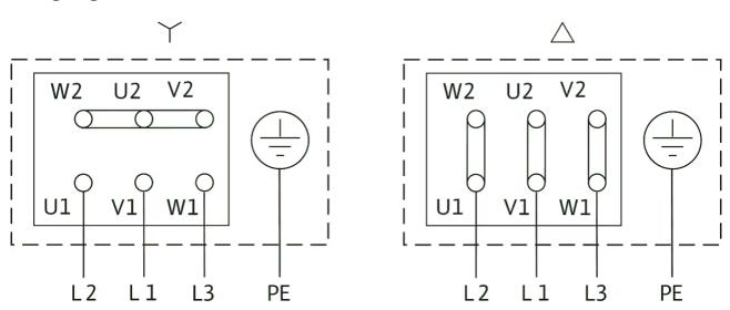
$\Delta$ : Connection diagram delta connection
