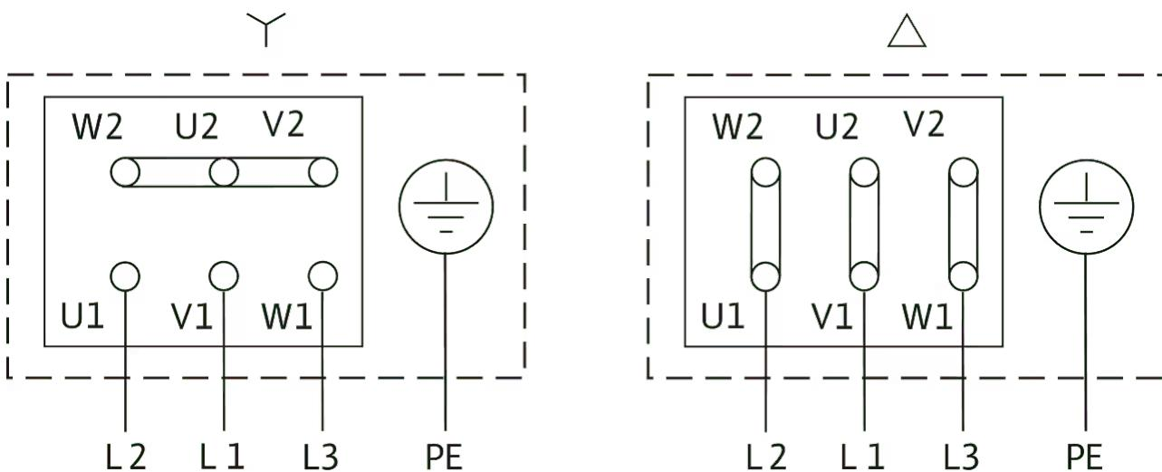
Δ: Connection diagram delta connection
