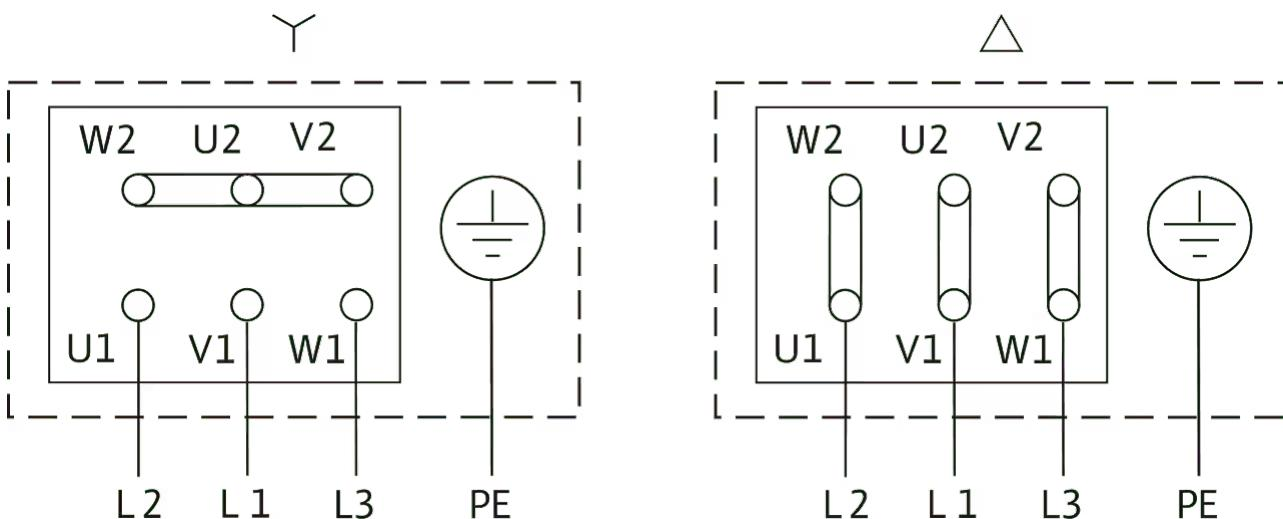
Δ: Connection diagram delta connection
