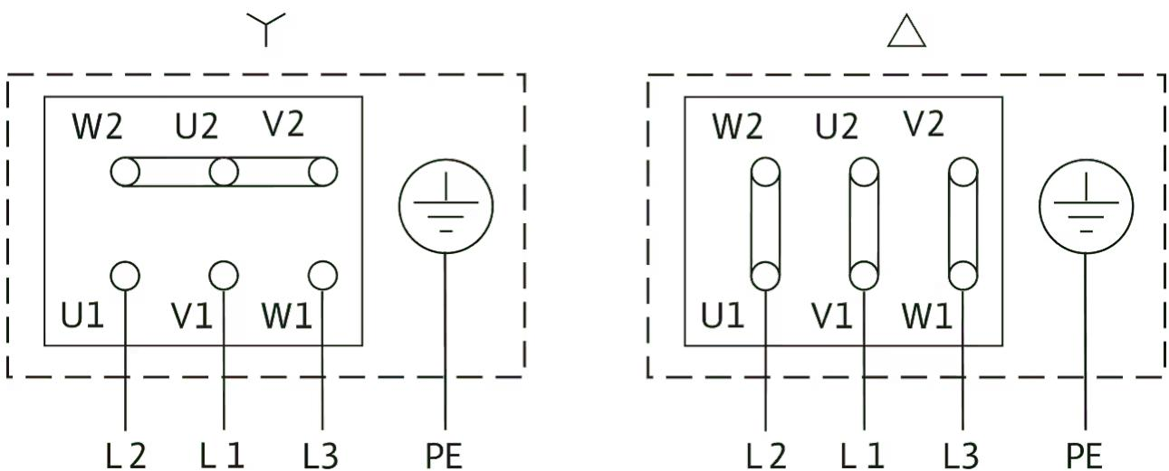
Δ: Connection diagram delta connection
