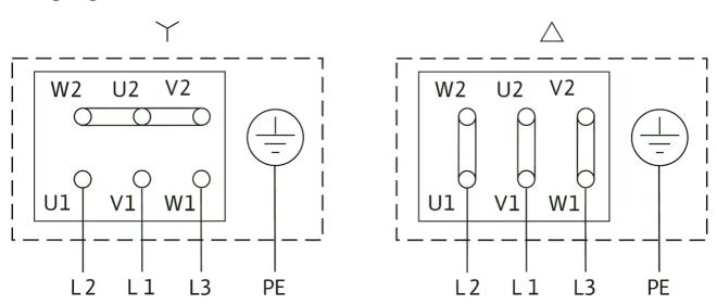
Δ: Connection diagram delta connection
