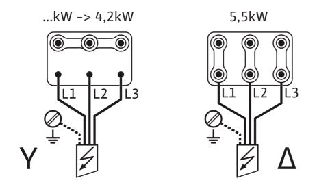
$\sim 3 400 V 50 Hz / \sim 3 380 - 460 V 60 Hz$
