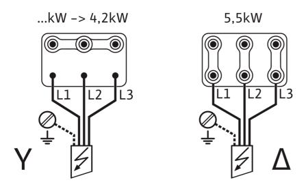
$\sim 3 400 V 50 Hz / \sim 3 380 - 460 V 60 Hz$
