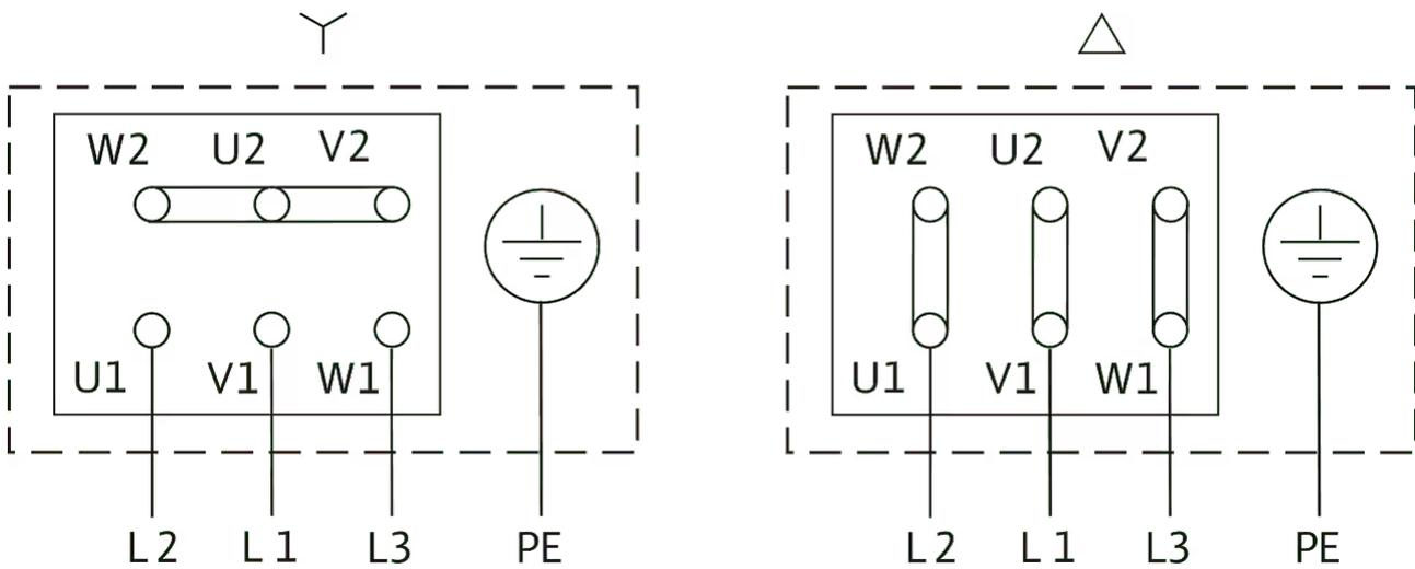
Δ: Connection diagram delta connection
