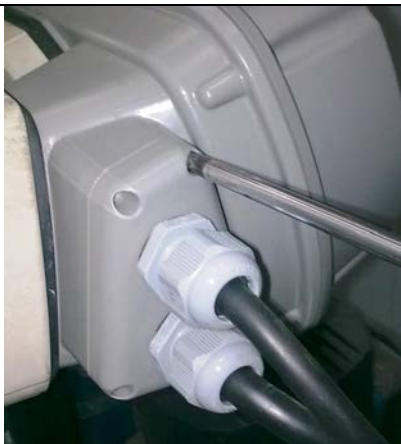
Open the side cover (4 screws)
