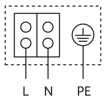
Blocking current-proof motor Single-phase motor (EM) 2-pole - 1~230 V, 50 Hz wilo
