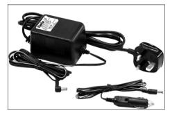
**NOTE:** A 5 amp fuse is fitted into the cigarette lighter plug adaptor, accessed by unscrewing the end cap of the adaptor. Take care not to loose the spring when unscrewing this cap.
