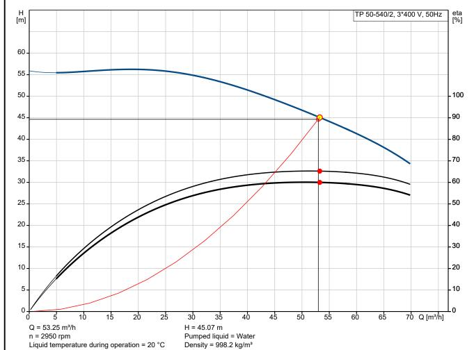
Eta pump = 65.2 % Eta pump+motor = 60 % NPSH [kW] [m] 35 14 P1 30 12. 10. 25 8. 20 6. 15 10 2. .5 P1 = 10.88 kW P2 = 10.01 kW
