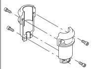
The motor stool connects the pump head and motor. The pump head has a combined 1/2" priming plug and vent screw.
