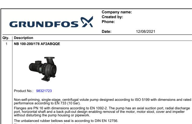
The pump is close-coupled to a fan-cooled asynchronous motor.
