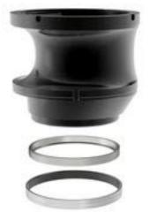
The shaft seal consists of two mechanical seals that ensure a reliable sealing between the pumped liquid and motor. The shaft seals are incorporated in a single-unit cartridge shaft seal system that is easy to replace in the field without use of special tools. The combination of the primary and secondary seals in a cartridge shaft seal system results in a shorter assembly length compared to conventional shaft seals.
