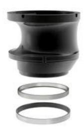
The shaft seal consists of two mechanical seals that ensure a reliable sealing between the pumped liquid and motor. The shaft seals are incorporated in a single-unit cartridge shaft seal system that is easy to replace in the field without use of special tools.
