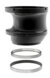
The shaft seal consists of two mechanical seals that ensure a reliable sealing between the pumped liquid and motor. The shaft seals are incorporated in a single-unit cartridge shaft seal system that is easy to replace in the field without use of special tools. The combination of the primary and secondary seals in a cartridge shaft seal system results in a shorter assembly
